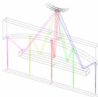
Figure 2: Polygon scanner optical schematic using non-spherical focusing mirrors
