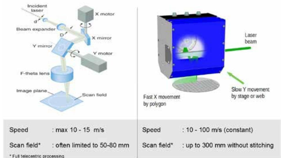
Figure 1: Galvanometer and polygon scanning techniques
