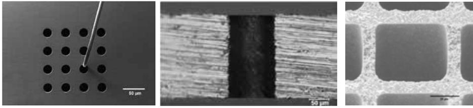
**Figure 6 left: array of bore holes machined in the precSYS's image field without xy-stage, middle: cross section of a zero tapered 100-µm bore hole, right: square hole array with aspect ratio 10 (Image, process development and processing by Posalux SA)**
