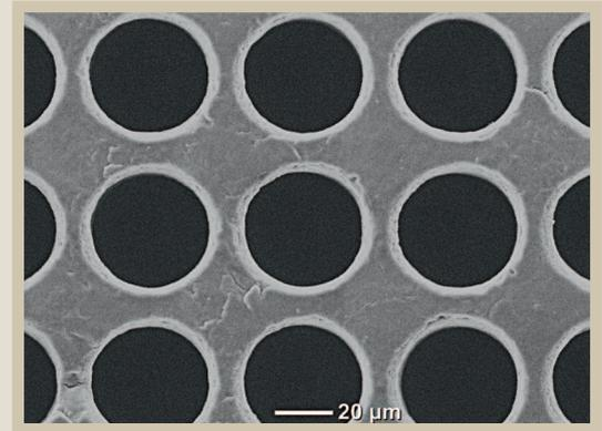
reliability within the Precsys subsystem's image field, round or rectangular holes with diameters and edge lengths up to 40 µm need to be fabricated while maintaining a 50 µm raster.
