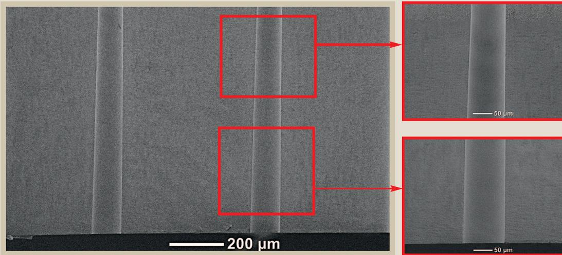
Figure 5. SEM (Scanning Electron Microscope) images of an injector bore hole, entrance diameter = 90 µm, exit diameter = 105 µm in a 1 mm thick wall
