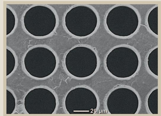
reliability within the Precsys subsystem's image field, round or rectangular holes with diameters and edge lengths up to 40 μm need to be fabricated while maintaining a 50 μm raster.
