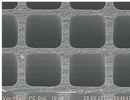
Figure 6. Square bore holes with an edge length of 40 µm, a 50 µm raster and a Si<sub>3</sub>N<sub>4</sub> substrate
