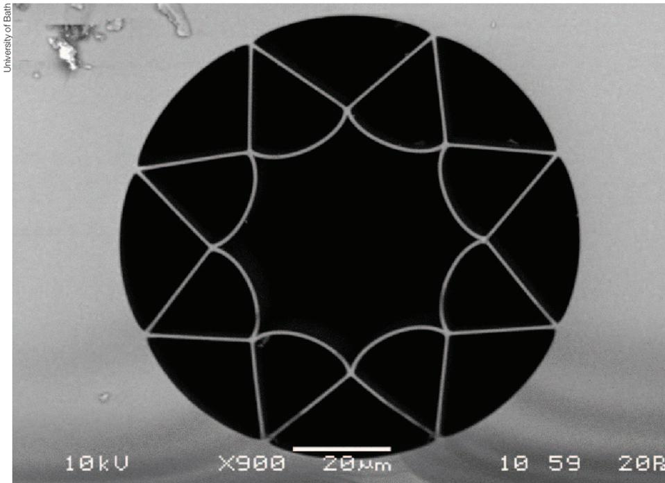
An SEM image of an anti-resonant fibre made by the University of Bath. The parts that appear black are air, and the rest is glass. The core guiding region is in the centre. The curved 'walls' surrounding the core are less than 1µm thick
