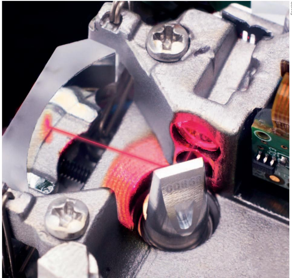
Scanlab's digital encoder technology in a galvanometer scanner, enabling it to meet future market needs
