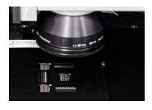
Until now, a scanner's image field has been the key limitation in laser processing – regardless of whether that entails marking, cutting, drilling or even microstructuring. Wide-area process tasks are executed step-by-step, by processing individual 'tiles'. This approach can involve relatively long process times and stitching errors, i.e. marking displacements at image field boundaries.
