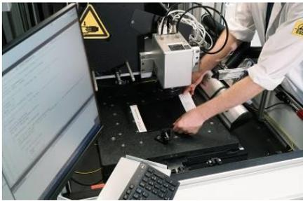
Laser processing is often constrained by a scanner's image field. Large-scale processing traditionally gets performed stepwise via individual image fields, called 'tiles'. But this method bears the risk of longer process times and stitching errors, i.e. misaligned marking at image field boundaries. To overcome this problem, SCANLAB and ACS Motion Control last year introduced a new scan concept. XL SCAN and
