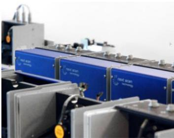
USP lasers are ideal for ultra-precise micro-machining of diverse materials, because cold ablation allows particularly fine, targeted material removal. To achieve industrial-scale productivity, USP lasers are best combined with ultra-fast scanners – e.g. a polygon scanner. In 2014, SCANLAB introduced its hybrid polygon scan system.
