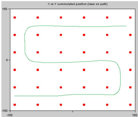
Fig 1 – Schematic representation of the stage path (green) and the simultaneous motion path (red) not true to dimensions and details
