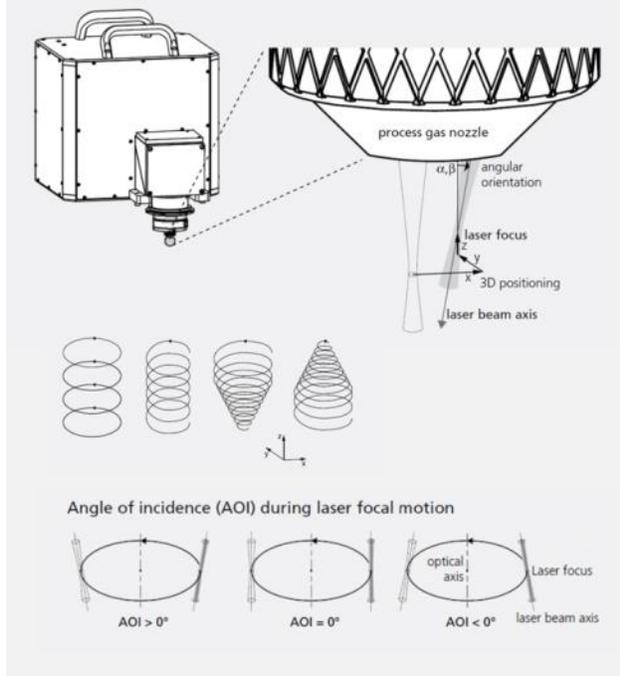
Fig 4 – System design for flexible laser processing in the  $\mu\text{m}$  range
