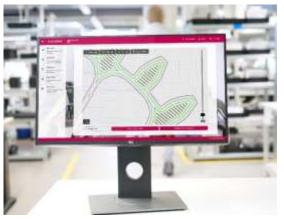
Additive manufacturing (AM) and especially metal AM strives for increasing throughput and less scrap. Data preparation is key to increase productivity and shorten process development times. The control system *SCAN*motionControl allows process developers to simulate the scan paths of the lasers offline on the PC. As the physical properties of the scan systems are taken into account in the simulation, the paths in the application are
