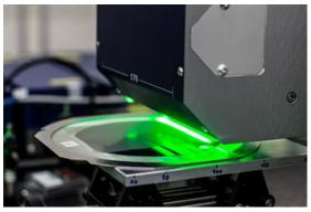
Polygon scan systems are renowned for their extremely high scan speeds, and are particularly well suited to line-by-line, flat laser processing of diverse materials. By using polygon scanners industrial productivity can be sped up in applications such as micro-structuring of touchscreens and solar cells or processing of electronic components.
