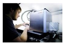
The robust precSYS 5-axis scan system was created for industrial volume production via ultra-short-pulse (USP) laser micromachining. The system enables fabrication of flexibly definable geometries, e.g. bore holes that are positively or negatively conical, ideally cylindrical, circular, rectangular or elliptical, as well as cavities with high aspect ratios and all with very good quality
