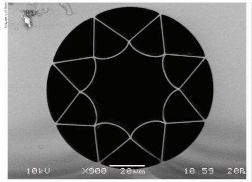
An SEM image of an anti-resonant fibre made by the University of Bath. The parts that appear black are air, and the rest is glass. The core guiding region is in the centre. The curved 'walls' surrounding the core are less than 1µm thick
