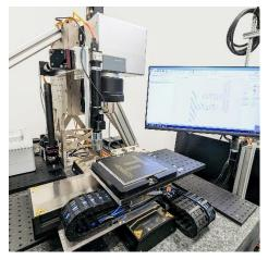
The XL SCAN solution can improve accuracy, feature resolution and throughput of micromachining of larger sized parts by synchronously controlling a 2D scan head and 2-axis XY stage motion. The scan solution incorporates the expert know-how from market leading scan systems with the long-standing experience of controlling mechanical axes. It provides highest precision within a virtually limitless working area, which is a key feature for various applications in electronics manufacturing.
