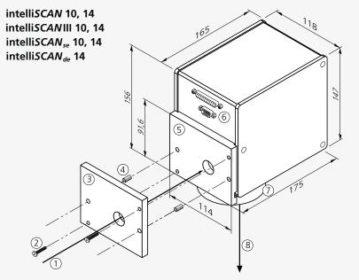
Denoted dimensions refer to the standard housing type (with standard mounting bracket). Variations in size and form are possible; also housings with water cooling have other dimensions.
